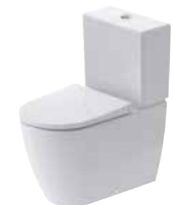
Set Toilet close-coupled Duravit Rimless® washdown model, outlet for Vario connector set, for horizontal and vertical outlet, length adjustable from 70 - 170 mm, and vario connecting bend, vertical outlet from 155 - 225 mm, UWL class 1. Toilet incl. seat & cover w/ soft closure
